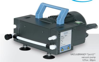
The Tyro12<sup>TM</sup> is an economical vacuum pump for a wide variety of laboratory tasks when budgets are a concern. Offering 15mbar (12Torr) ultimate vacuum and 35lpm (1.2cfm) free air capacity, the Tyro12<sup>TM</sup> is suitable for rotary evaporation, gel drying, and many
