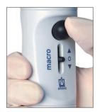
**Blow-out function** When using blow-out pipettes, press the convenient blowout bulb once the meniscus has come to rest in the pipette tip. Pipetting has never been easier.
