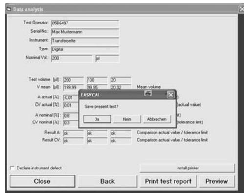
In case the instrument is tested for the first time you will be asked at which interval the instrument has to be tested again. Please enter the required interval in months (1-99).
