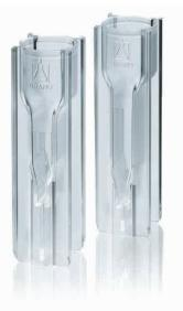
BRAND ultra-micro UV-Cuvettes. 15mm (left) and 8.5mm (right) window heights
